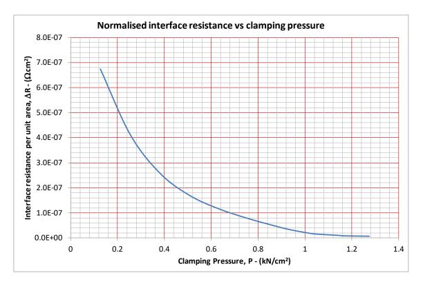
Figure 4 Normalised interface resistance variation with clamping pressure
