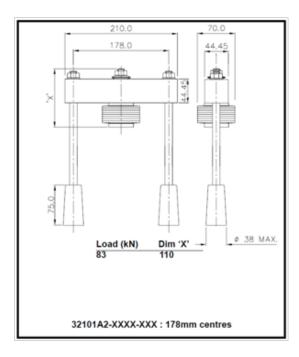
Figure 5 Typical Clamp for Double Side Cooling
