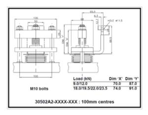
Figure 6 Typical Clamp for Single Side Cooling
